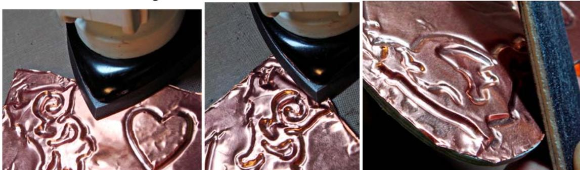
10. Use the emery file to carefully file the metal edges down around the sides of the cover. This will help with the edges adhering to the cover and not coming undone with wear. If necessary, reheat edges to activate glue to assure all edges are glued down.
